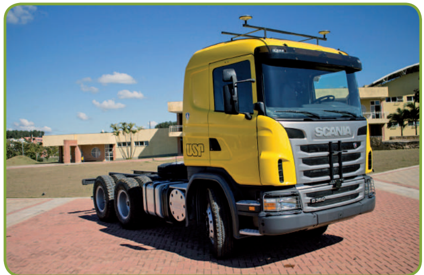
FIG 2 Autonomous truck developed in cooperation with Scania Latin America.
