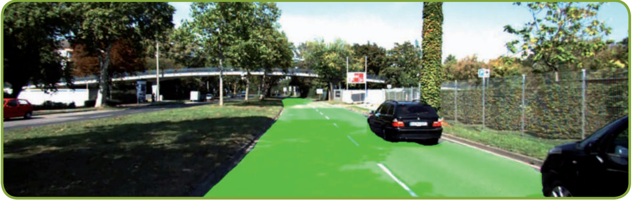
FIG 3 Road detection using convolutional neural networks.
